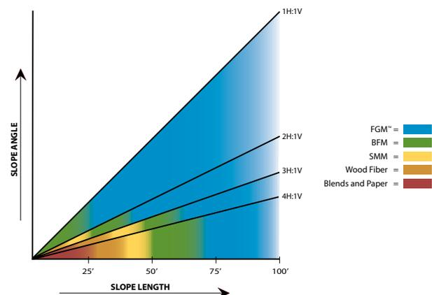
FIGURE 1: Hydraulically applied erosion control materials selection guideline
