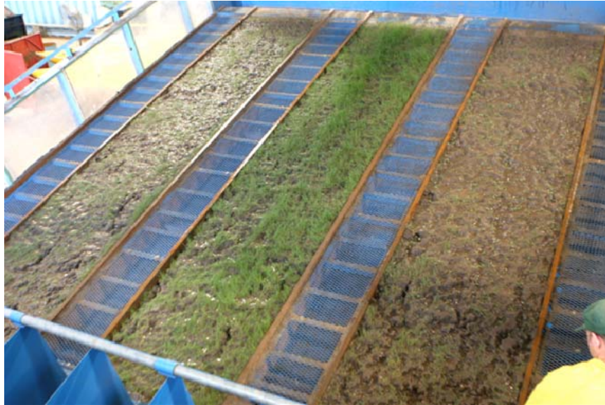
• Figure 6: : Bare Soil Control (left), Thermally Refined (center) and Hammer-Milled (right) Wood Fiber Mulches after the Plant-Establishment Period and Just Prior to the Post-Vegetation, 30-Minute Rainfall Event
