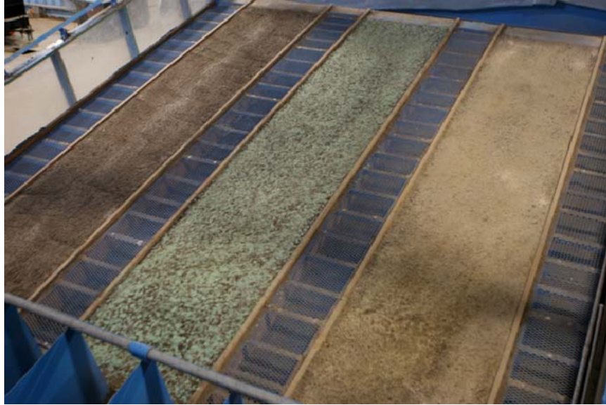
• Figure 4: Bare Soil Control (left), Thermally Refined (center) and Hammer-Milled (right) Wood Fiber Mulches Prior to the Pre-Vegetation, 30-Minute Rainfall Event.
