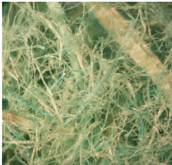
• Figure 3: Photograph of Thermally Refined Wood Fibers at 20 Times Magnification Through a Stereoscope
