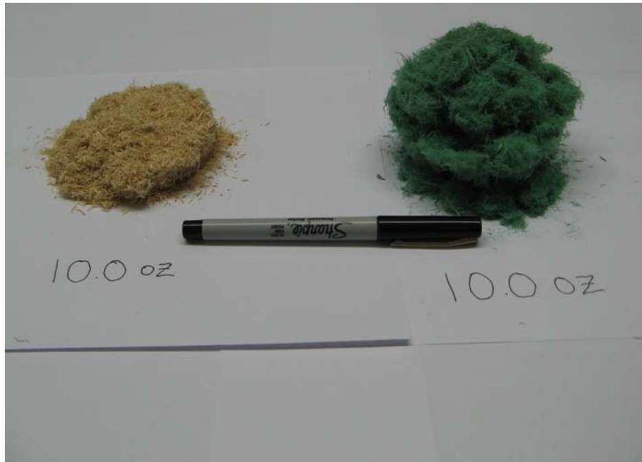
• Figure 1: Photograph of Hammer-Milled Wood Fiber (left) and Thermally Refined Wood Fiber (right) – 283.5 grams of each
